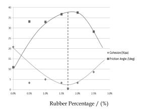
Figure 1: Variation of Cohesion and Friction angle with rubber content
