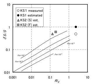
Figure 6 Present and future conditions of Koggala lagoon in Fisher diagram. ○, measured salinity difference;●, ▲ and ■, estimated value based on *Ri<sub>E</sub>* and *Fm*
