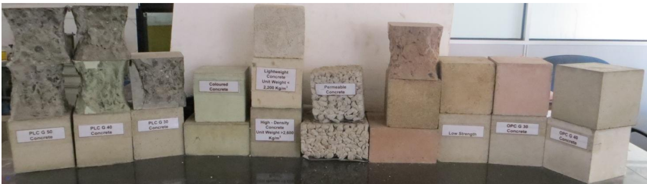
Figure 4: Different types of concrete tested at Holcim Lanka Innovation & Application Center (Pervious, light weight, Low strength, high strength, coloured etc...)
