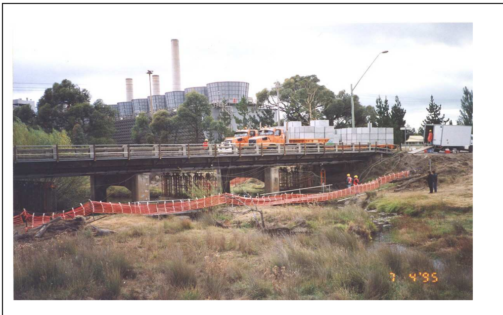
Figure 17 – 1st Proof Load Testing (1995)
