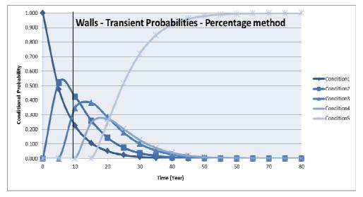
Figure 4: Transient probabilities derived from condition data
