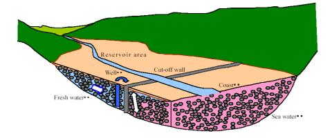
Fig – 12 Schematic diagram of underground dammed aquifer
