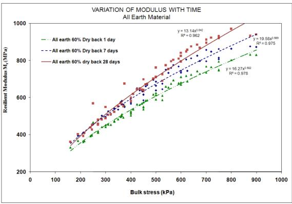
Figure 6: All Earth resilient modulus at 1, 7 and 28 days.
