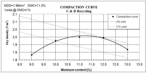
Figure 1: C & D Recycling compaction curve.
