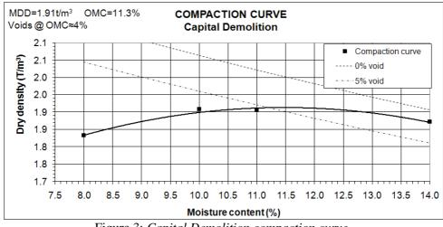
Figure 3: Capital Demolition compaction curve.
