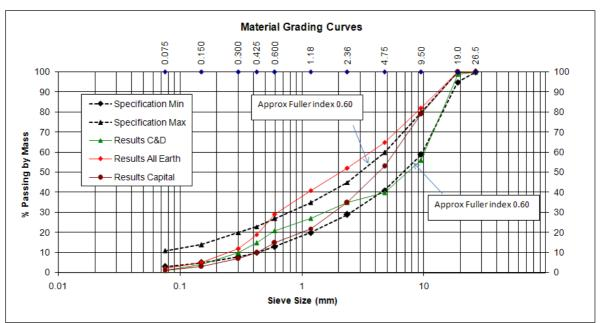
Figure 4: Particle size distribution for recycled materials.
