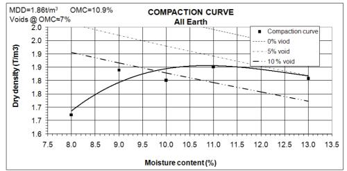
Figure 2: All Earth compaction curve.
