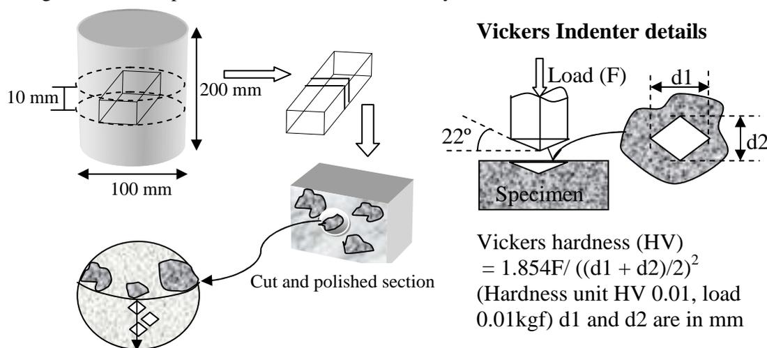
Fig. 1 Configuration of the Vicker's microhardness
