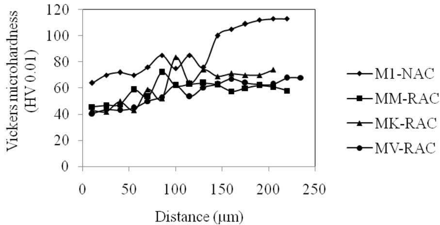
Fig. 3 Gradients of Vickers microhardness of both normal and recycled aggregate concretes
