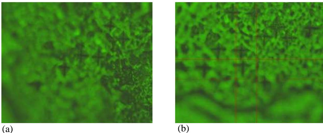
Fig. 2 Microhardness indentations (a) normal concrete (M1-NAC) and (b) recycled aggregate concrete (MM-RAC)
