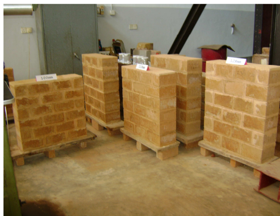
Figure 2 - Test panels constructed for testing
