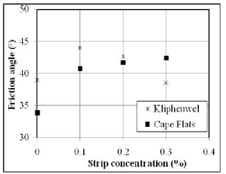
Figure 3. The friction angle versus reinforcement concentration
