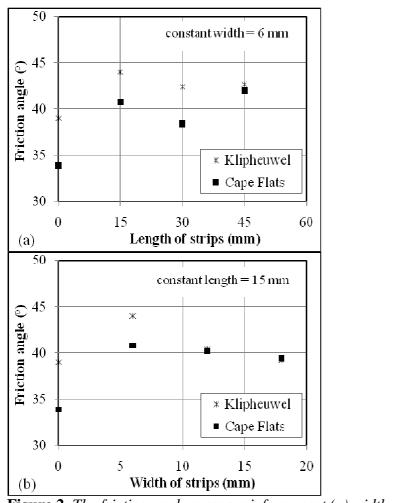
Figure 2. The friction angle versus reinforcement (a) width, and (b) width
