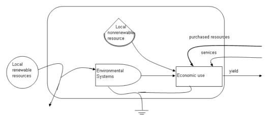
Figure 1. Diagram illustrating the production process by emergy flow diagram (from Ulgiati and Brown 1997).
