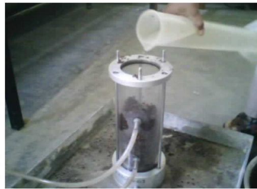
Figure 6: Sample preparation (a) application of small compaction and (b) addition of water
