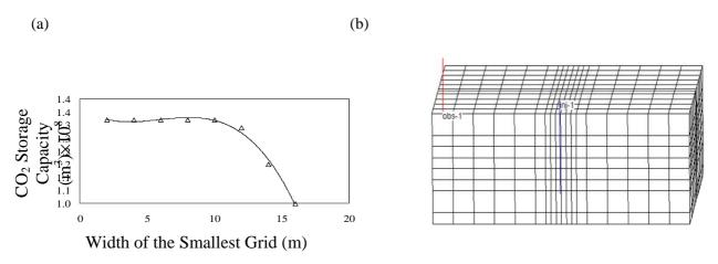
Figure 2. (a) Effects of grid size on storage, and (b) selected model grid blocks for the coal seam.
