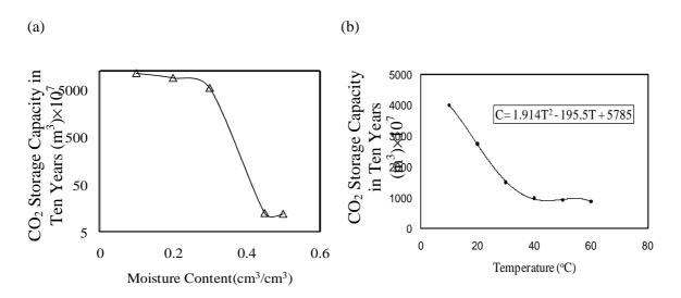
Figure 6. Variation of  $CO_2$  storage capacity of coal mass for 10 years of injection with the (a) coal bed moisture content and (b) coal bed temperature.
