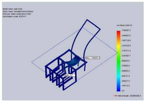
**Figure 9:** *Static nodal stress of the main body frame* Hence there was no excessive static nodal stresses developed in the main body as the test shown in above figure 9. The test was done by using solidworks
