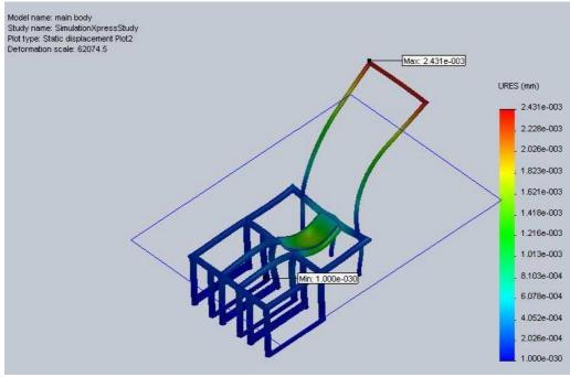
Figure 8: Static deflection of the main body frame
