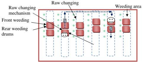
Figure 4. Top view of the Operational behavior in the field.
