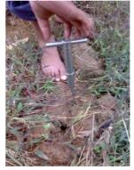
Figure 10: Vane shear testing
