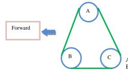
A– Driving wheel which connect to the intermediate shaft B & C–Driven wheels which connect to the weeding drums
