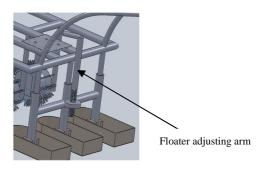
Figure 7: The floating mechanism
