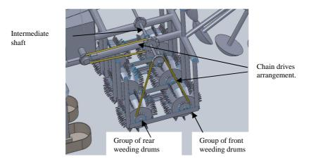
Figure 2: Arrangement of the weeding drums
