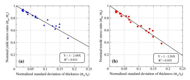
Figure 6: Relationship of (a) yield stress ratio, (b) tensile stress ratio and normalized standard deviation of thickness ( $\sigma_{st}/t_0$ )
