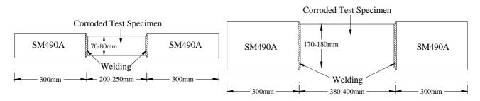
Figure 1: Dimensions of test specimens
