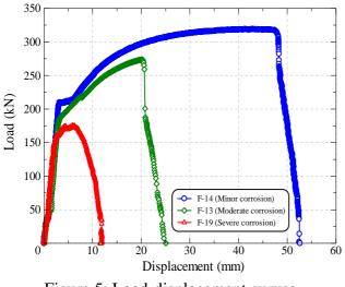
Figure 5: Load-displacement curves
