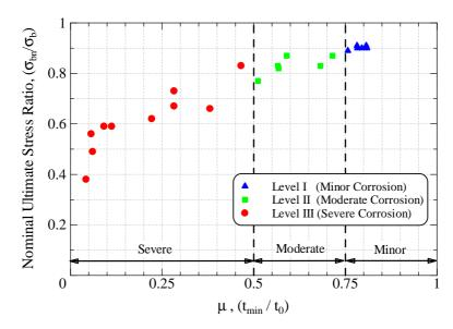
Figure 3 Relationship of ultimate stress ratio & minimum thickness ratio (µ)
