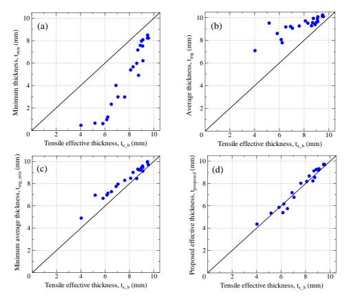
Figure 7: Relationship of (a)  $t_{min}$  vs  $t_{e_{-b}}$ , (b)  $t_{avg}$  vs  $t_{e_{-b}}$ , (c)  $t_{avg_{-min}}$  vs  $t_{e_{-b}}$  and (d) proposed effective thickness  $(t_{eff})$  vs  $t_{e_{-b}}$
