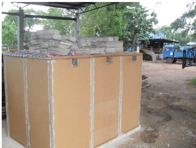
Figure 3: The load testing carried out for Dura panels with full scale model
