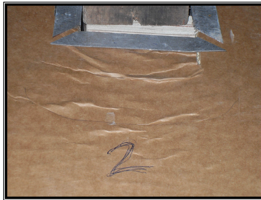
Figure 7: The localized failure suffered by the straw bonded solid panel
