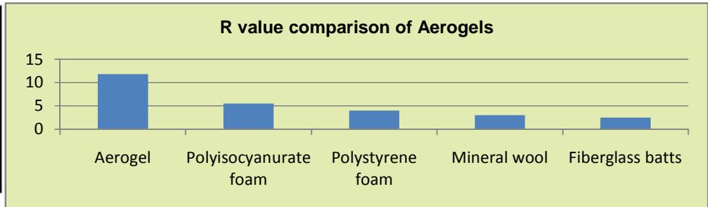
**Fig. 9:** R value comparison of Aerogels (Elvin, 2007)
