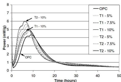
**Fig. 4:** Rate of Hydration of TiO<sub>2</sub> –blended cements (Jayapalan et al., 2009)
