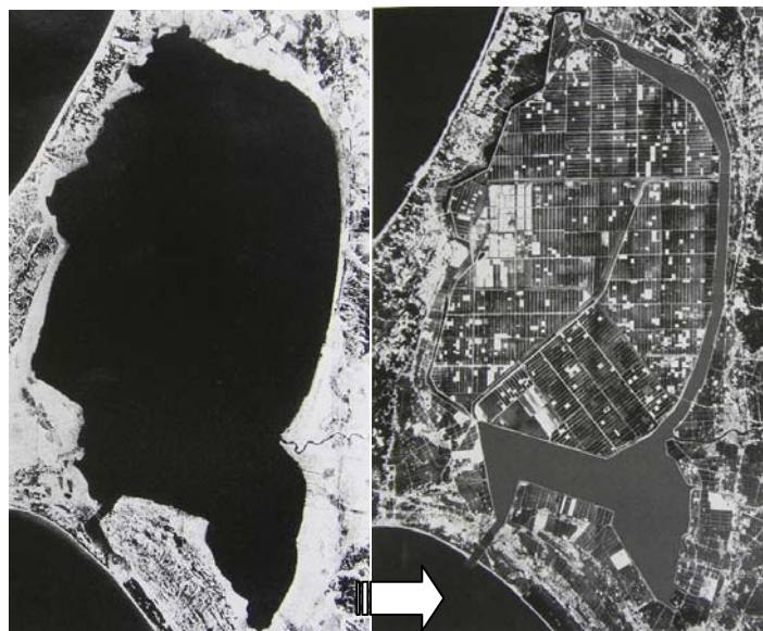
Figure 1: Land reclamation of wetland at second large Hachirou-Gata lagoon lake, where Changed to paddy field about 88% (Akita, Japan)
