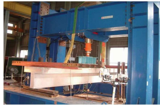
Figure 4: Test Rig Setup of Strip Foundation
