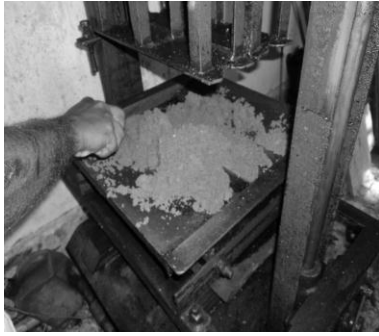
Figure 9: filled the mould with mortar
