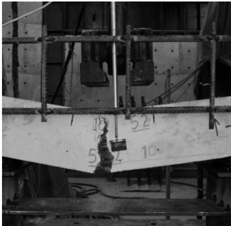
Fig. 11: Failure of polymer fibers as well as pull out effect of steel fibers
