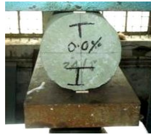
Figure 5: Test Setup for Splitting Tensile Strength
