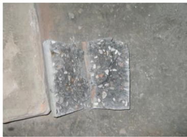
Figure 11: Brittle failure of specimen T_1
