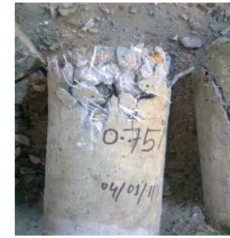
Figure 9: De-bonding of fiber-matrix of specimen C_4
