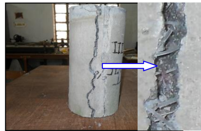
Figure 12: Fiber bridging of specimens T_2 , T_3 and T_4
