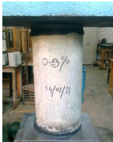
Figure 3: Instrumentation of Cylindrical Specimen to Test the Compressive Strength
