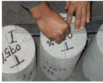
Figure 4: Marking the Cylinders in Progress
