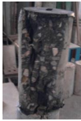
Figure 7: Brittle failure of specimen C_1
