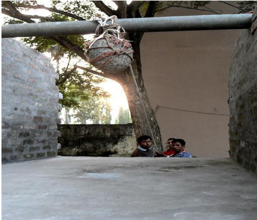
Figure 11: Impact test setup with round hammer ball, 1m free fall on slab
