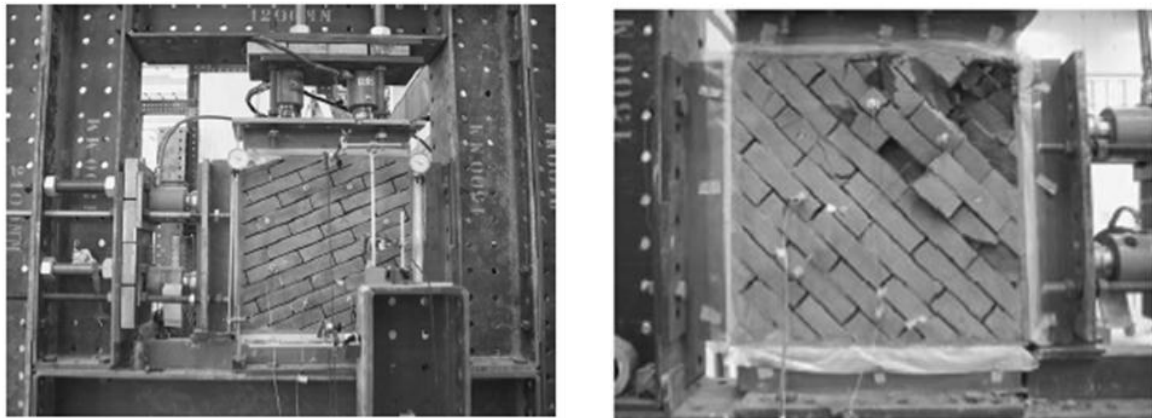
Fig 3: (a) Biaxial test rig of thin bed masonry (b) failure of panel in biaxial compression Vermeltfoort (2005)
