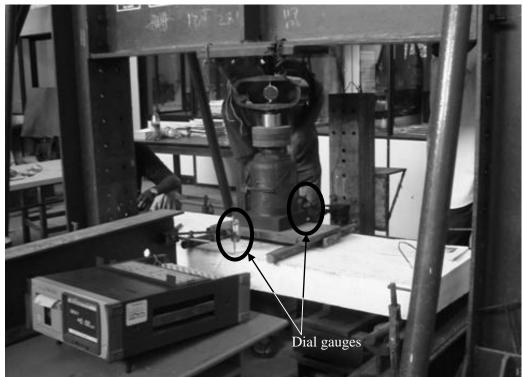
Figure 5: Test arrangement
