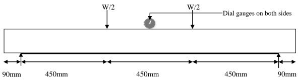
Figure 1: Slab loading pattern
