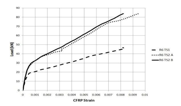
Figure 6: Load versus CFRP strain at mid-span relationship.
