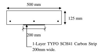
Figure 2: T10 - TS1 Cross section
