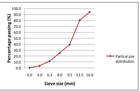
Figure 7- Particle size distribution of crushed coconut shells
