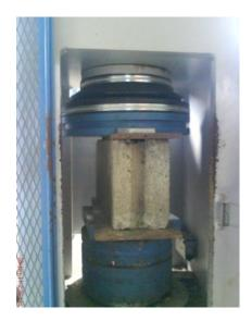
Figure 6-Testing of masonry block in crushing machine
