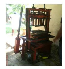
Figure 4-Local block manufacturing machine
