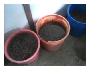
Figure 3-Saturation of the crushed coconut shell
