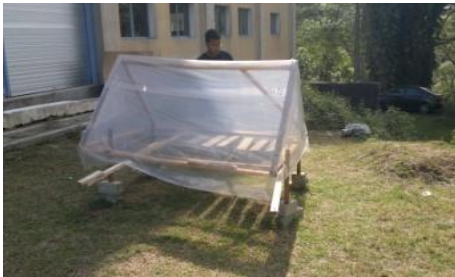
Figure 4: Specimens are intersected to rain only (In this arrangement the prisms are kept as its any side does not block the evaporation.)
