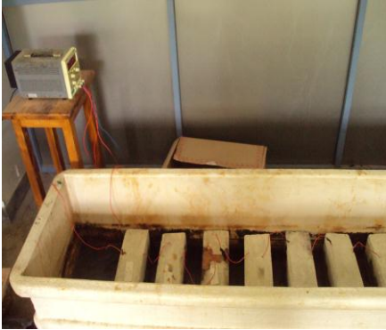
(a) Specimens under Acceleration Corrosion Testing at the Laboratory
