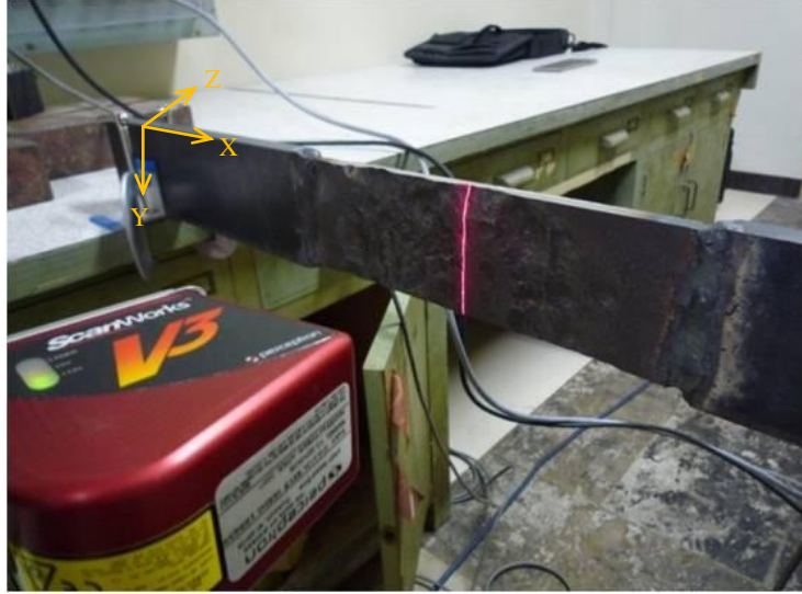
Figure 2: Condition of thickness measurement
