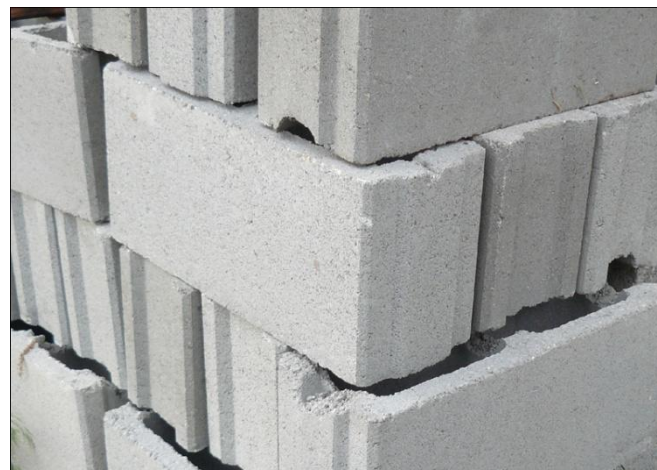
[Figure 1.b], Concrete block
