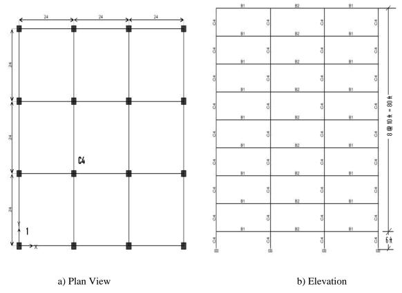
Figure 1 Plan & elevation of the hypothetical structure
