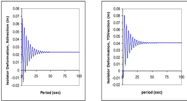
Figure 3 Isolator deformations in x and y direction due to time history loading
