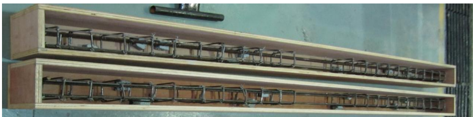
Figure 2: Appearance of the RC and SFARC beams before casting
