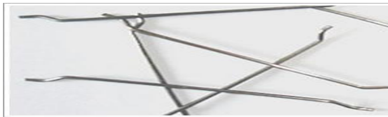
Figure 1: Hooked-end shape steel fibers used in this Study
