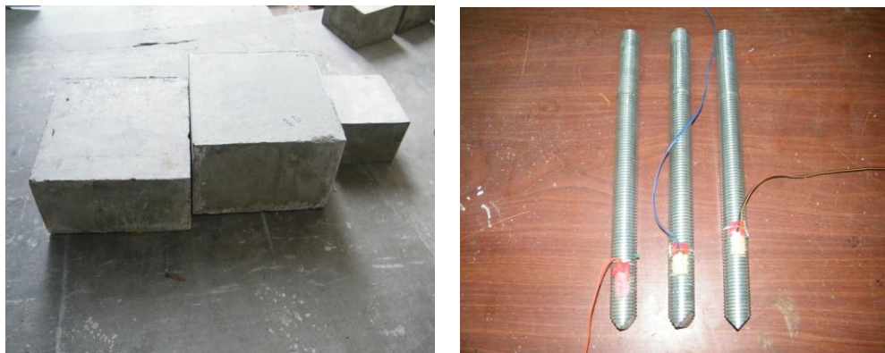
Figure 1. Concrete specimens, anchors and mounting of strain gauges.
