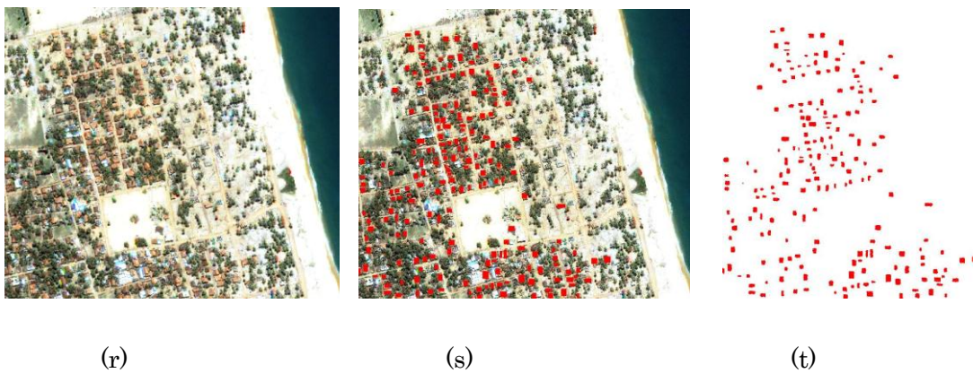
Figure 6. Building extraction results. (r) IKONOS image of the post-tsunami area. (s) Manually labeled buildings as ground truth. (t) Result of the building extraction according to approached method.
