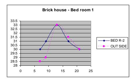
Chart 1: Indoor and outdoor temperature in brick house with clay tile roof
