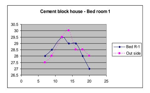
Chart 2: Indoor and outdoor temperature in cement block house with cement fiber roof
