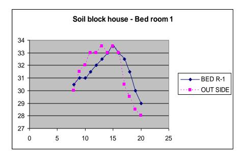
Chart 3: Indoor and outdoor temperature in soil block house with MCR tiles
