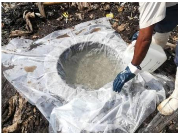
Figure 3-7: Determination of in-situ density
