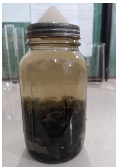
Figure 3-8: Pycnometer with waste sample and water
