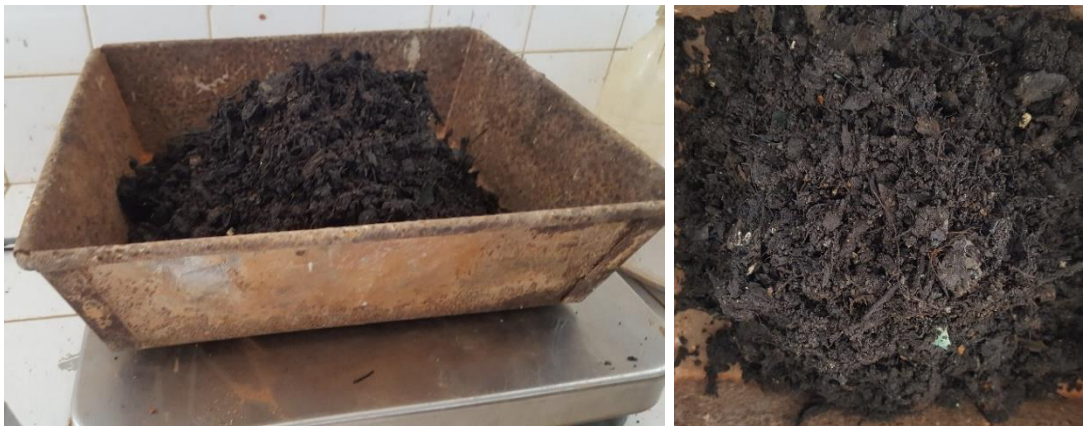
Figure 3-3: Sample 1 obtained from the bottom of the waste fill
