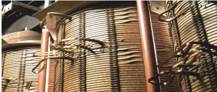
Figure 2.2 Paper insulation of Transformer [3]
