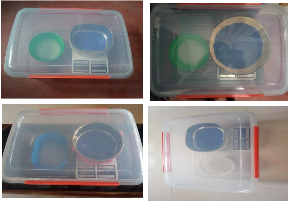
Figure 4.2 Experiment arrangement at 75% relative humidity [26],[27]
