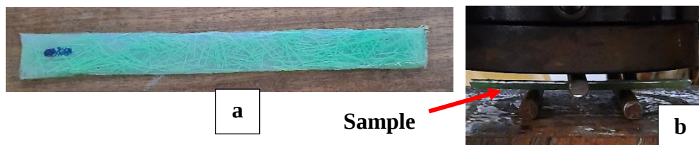
Figure 4.16 – (a) Flexural strength testing sample (b) Testing a sample
