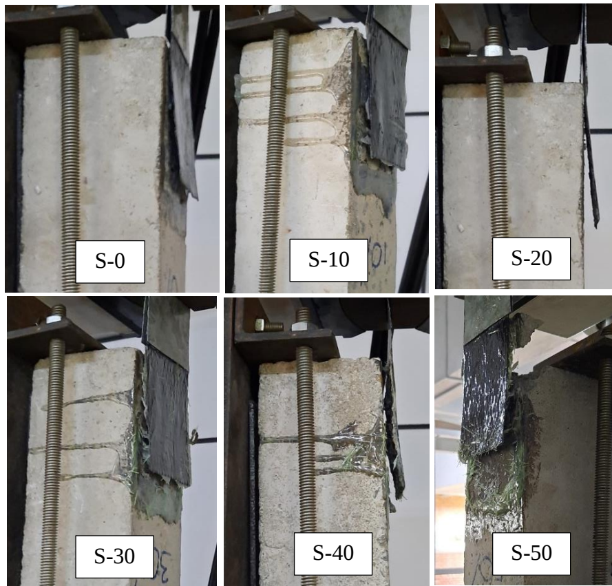
Figure 4.4 – Debonding failure occurrence
