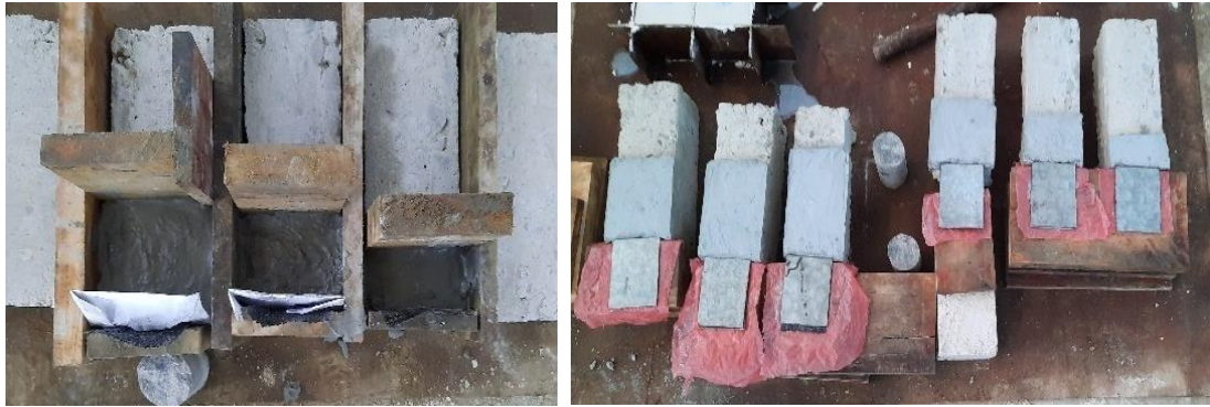
Figure 3.8 – Preparing samples for direct pull out test
