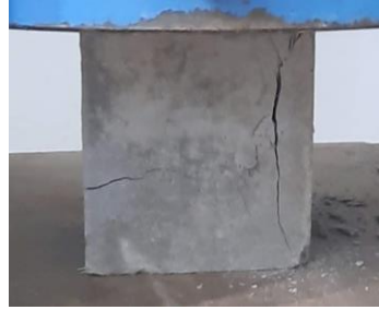
Figure 5.10 – Testing the compressive strength
