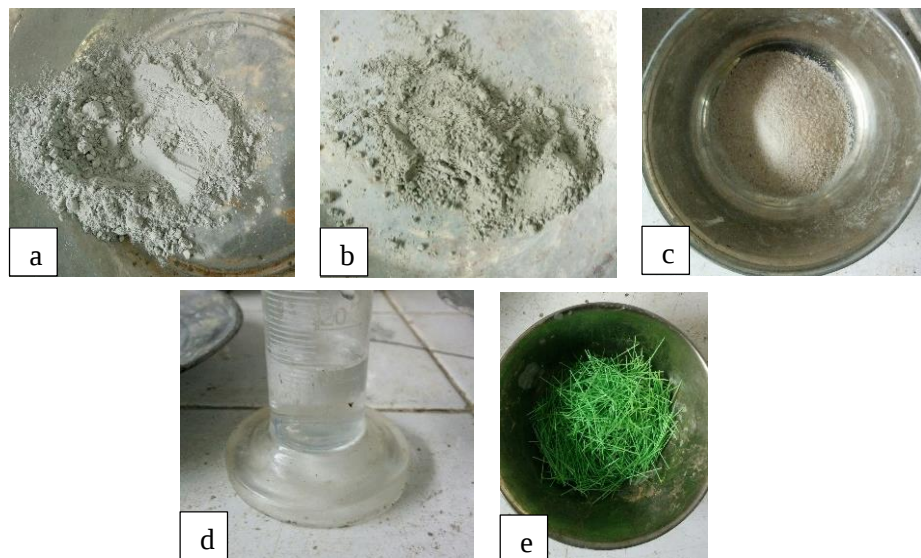
Figure 3.1 – Materials used to develop ECC adhesive, (a) Portland cement (b) Fly ash (c) Silica sand (d) Water (e) PET fibers
