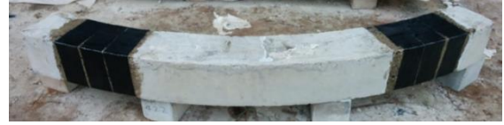
Figure 1(b) CFRP strengthened beam
