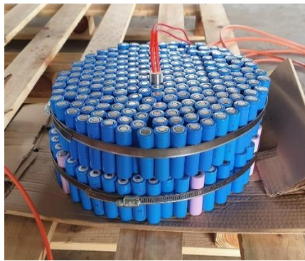
Figure 4-4: LIB bundle, worm-screw clamps and ignitor
