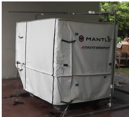
Figure 5-14: AKE CFCC post-test
