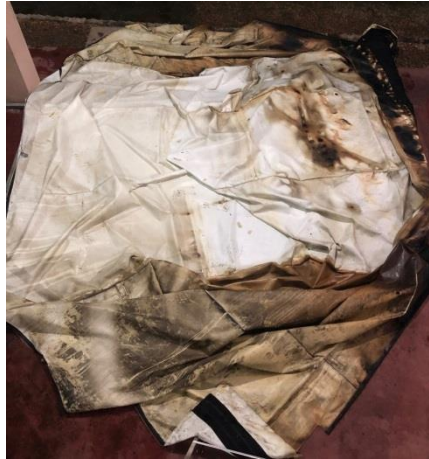
Figure 5-7: Post-test interior condition of AMJ CFCC
