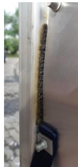
Figure 5-11: AKE container side damages
