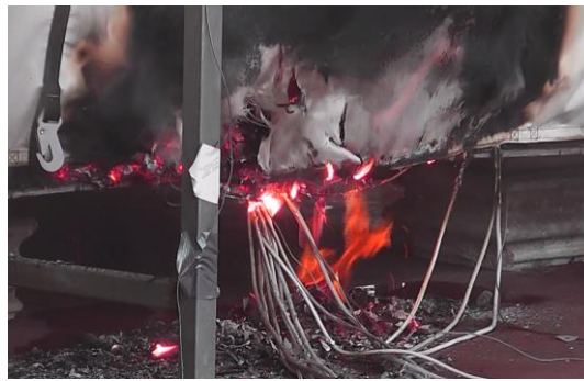
Figure 5-3: Fabric failure in phase 2
