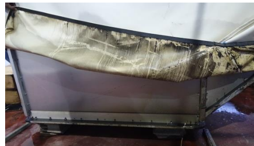
Figure 5-15: AKE CFCC fabric inner side discolouration
