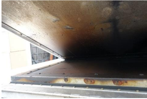
Figure 5-12: AKE container slanted edge damages
