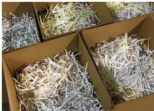
Figure 4-7: Class A load - boxes and shredded paper
