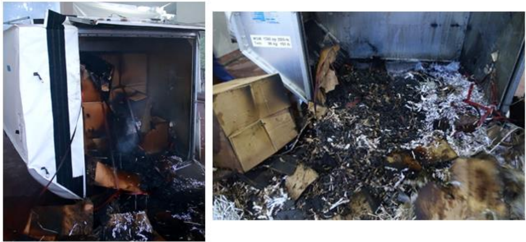
Figure 5-9: Post-test observations of AKE container
