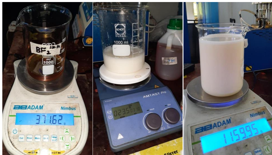
Figure 3-1: Base fluid preparation; [a]- Preparing of PGPR and TWEEN 80 mixture; [b]- Adding coconut oil into the pre- prepared mixture and stirring; [c]- Adding water into pre- prepared mixture
