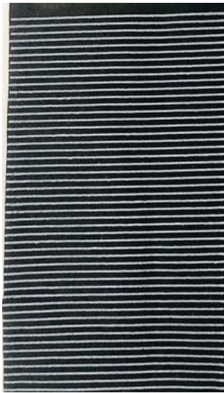
Figure 12- 1.0mm between two glue dot lines
