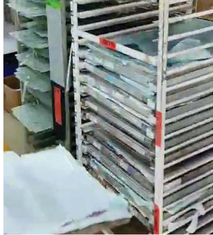
Figure 17 - Racks for panel curing
