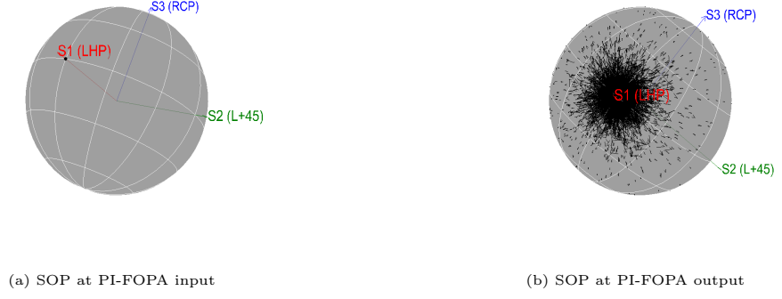
Figure 4.4: Poincare sphere representation of the input SOP variation at the output of PIA
