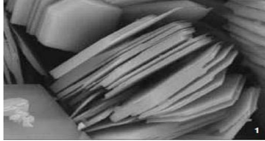
Figure 2.5: Hexagonal crystal structures (Bloomfield, 2016)
