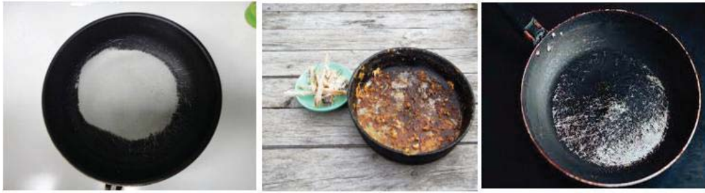
Figure 2.1: Damaging of nonstick layer of nonstick metal cookware (Shimizu et al., 2012)
