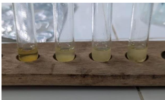
Figure 6. Obtained precipitations after conducting the iodoform test.
