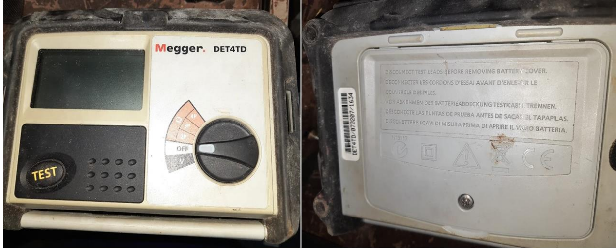
Figure 40 : Equipment used for earth resistance measurement
