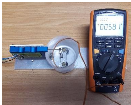
Figure 5.17: Experimental Setup (a) SMA Spring Attachment with Force Measuring Apparatus; (b) Measuring Temperature through the Thermocouple Probe
