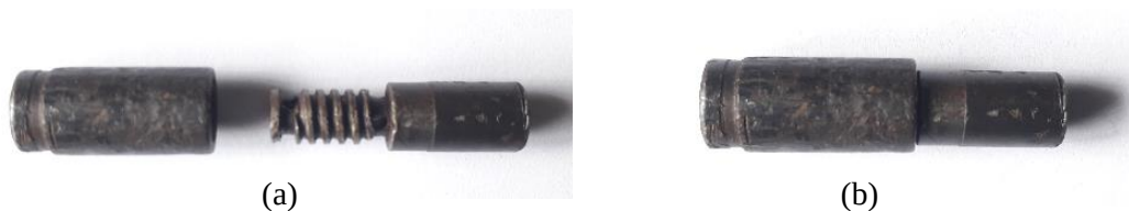
Figure 4.5: Spring Forming Fixture (a) Fabricated Fixture and Sleeve; (b) Assembled Fixture
