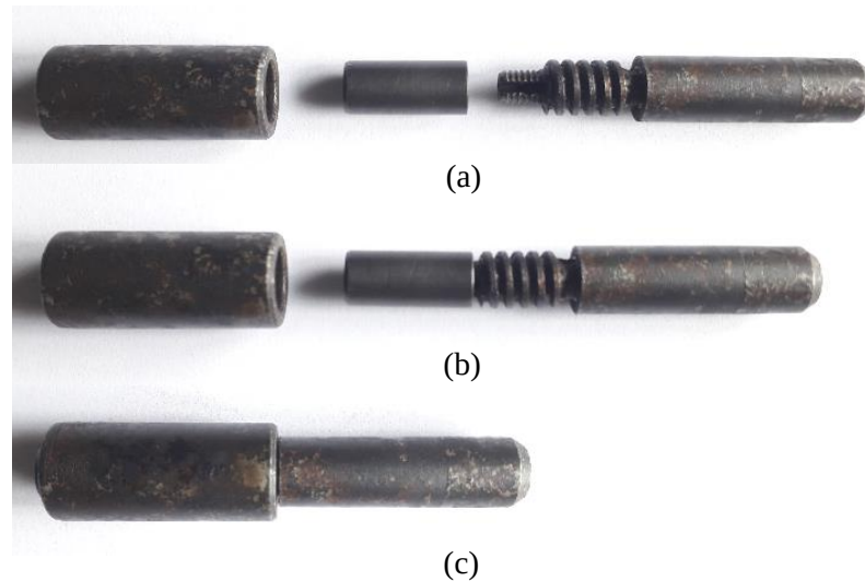
Figure 4.7: Modified Fixture (a) Fabricated Sleeve, Positioner and the Fixture; (b) Positioner Assembled with the Fixture; (c) Assembled with the Sleeve
