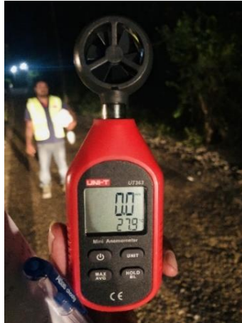
Figure 5: Measuring of wind velocity & air temperature a digital anemometer with thermometer
