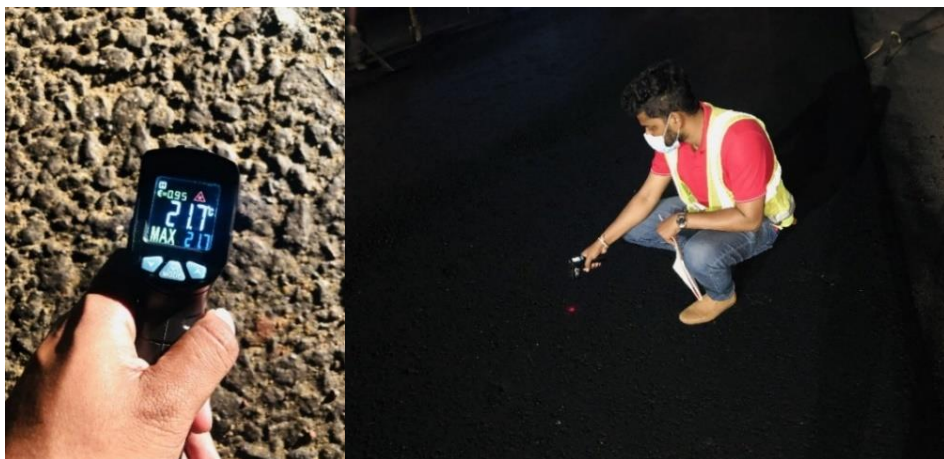
Figure 4: Measuring of base temperature using an infrared thermometer
