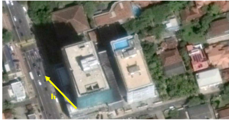
Figure 6.15: Building Height Based on the Image Shadow
