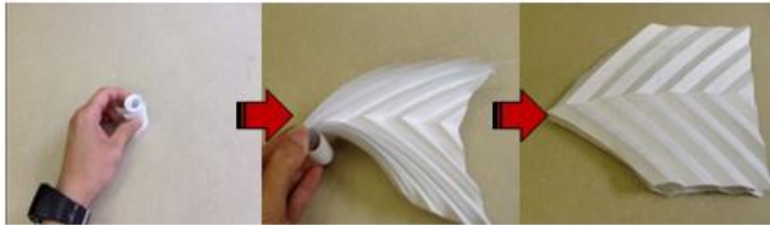
Curved beech leaf crease pattern - Initially wrapped to intermediate stage to final deployment
