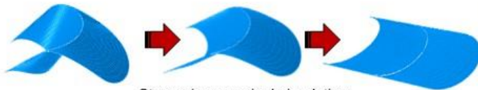
Stages in numerical simulation - Fully folded to intermediate stage to final deployment
